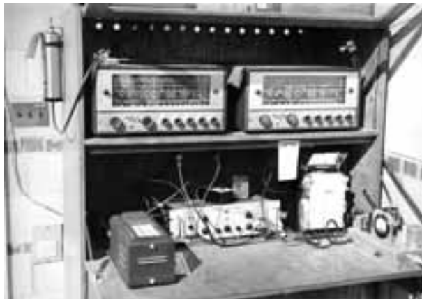
Figure 2: The receiving equipment. The second receiver was used for time signals from WWV. The noise generator is on the extreme right-hand side.
