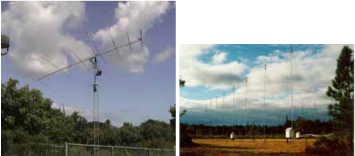
Figure 2: The 17–30 MHz steerable log periodic antenna in Hawaii (left) and the 16–element 18–30 MHz TP Array at the University of Florida Radio Observatory.
