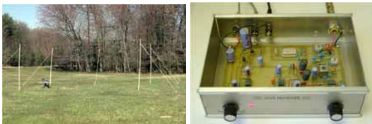
Figure 1: The standard Radio JOVE Double Dipole Antenna and 20.1 MHz RJ1.1 Receiver
