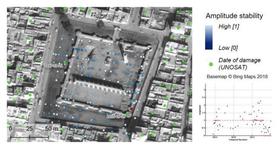
Figure 6: Amplitude stability of PS at the Great Mosque of Raqqa. The amplitude series of the location is marked in red, bottom right. The damage identified in the UNOSAT data is indicated in green, with selected dates. Note that the basemap image was taken before the civil war.
