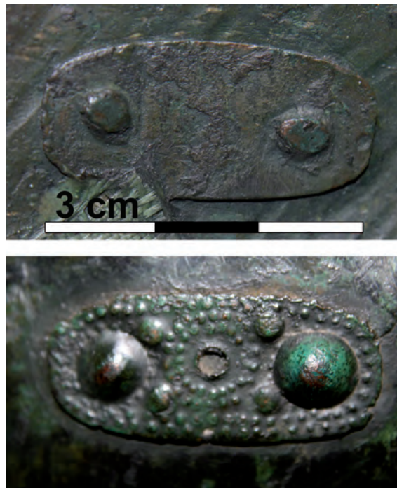
Fig. 2.6 Helmet of Type Pişcolt from the eponym find spot in Romania. Details of the riveted on decorated bronze on the outside of the helmet (below). On the inside, another sheet was applied (above). The overlapping hammering traces indicate that it was applied during the manufacture process.
