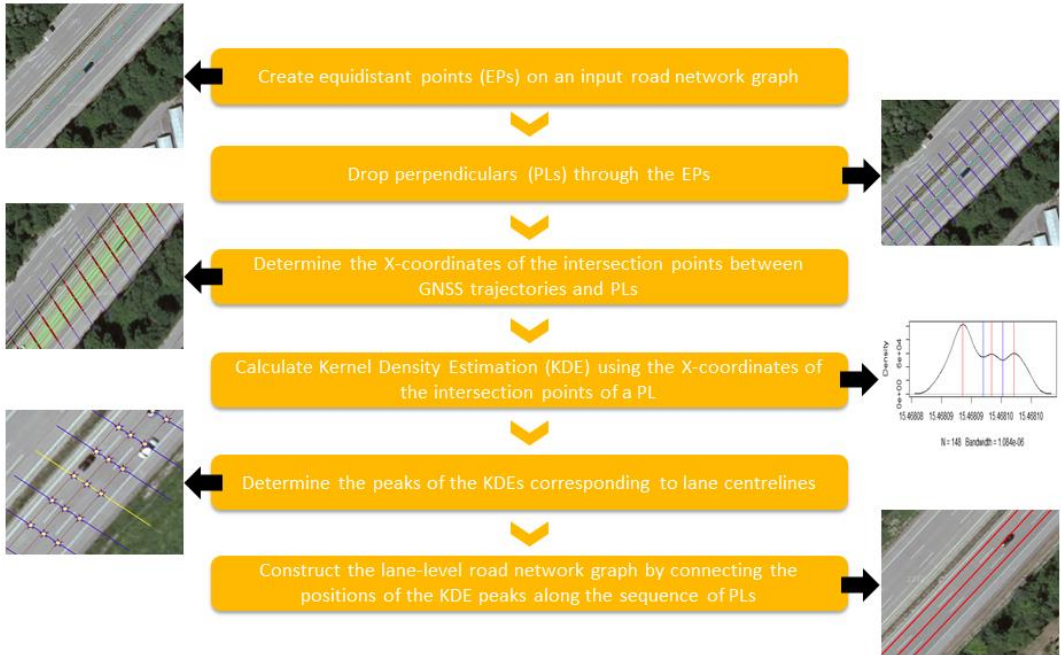
Figure 3: Main processing steps for deriving the lane-level road network graph
