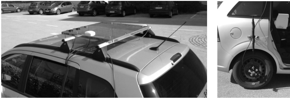
Fig. 2: Placement of the sensors: Demagnetized steel plate and porcelain antenna (left) for the GNSS observations and car-mounted CORRSYS (right) to track the wheel rotation.
