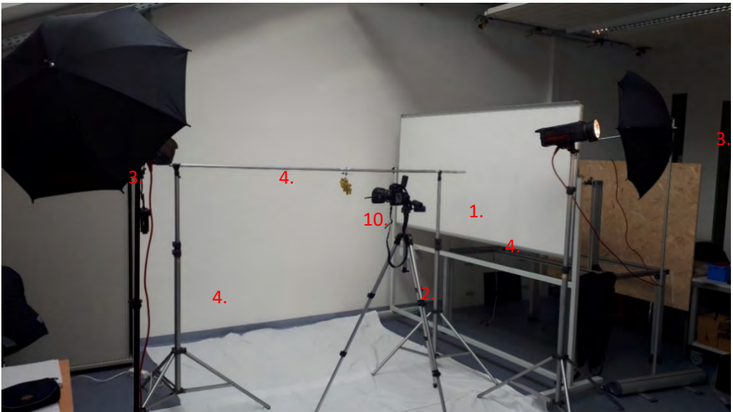
Figure 2: Data capture construction: 1. Camera, 2. Tripod, 3. Flashers, 4. Bars, 10. Grapes
