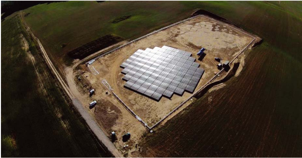
Figure 6: The LOFAR station in Baldy. LBA field (right), HBA field (left).
