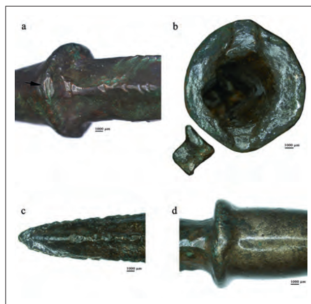
Fig. 4. Evidence of production in two-part casting mould of knives. – a. Casting seam remains on INZ 9/6. – b. Casting seam remains and detail of mismatch in tang section in FHK 40/5. – c. Casting seam remains on tang tip of FHK 444/4. – d. Mismatch in intermediate section of FHK 444/4 (Photos: N. Mittermair).
