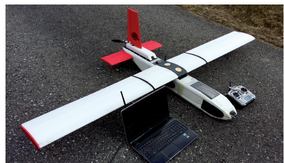
Figure 1 – The equipment used: Maja-D drone, a laptop containing a telemetry link as ground station, and the remote control. © S. Weber
