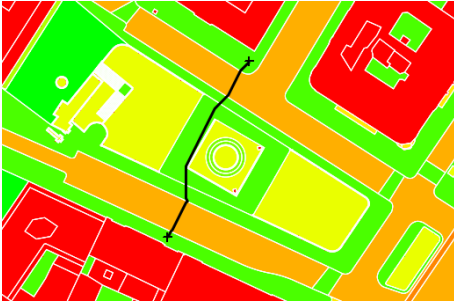
Figure 3: Least-cost path over a cost surface (colours from green = low cost, to red = extremely high cost); example using GRASS GIS r.walk at Dr.-Karl-Lueger-Platz, Vienna
